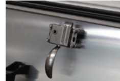
L01 Internal Cablock
